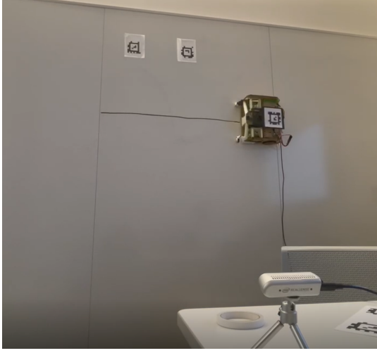
Fig. 2: Experimental setup showing WIPER mounted on the whiteboard with AprilTag markers for localization and an Intel RealSense D435 camera for visual tracking. The cable provides power and data connectivity during testing.
